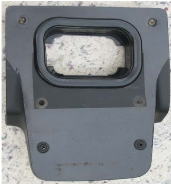
Figure 4. Grommet installed in hole.
