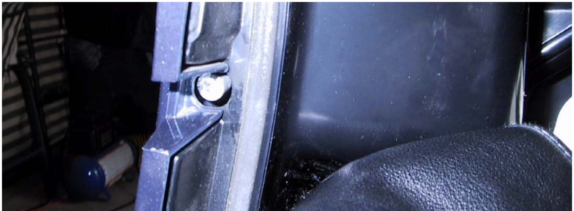
Figure 10. Taillight assembly bolt for 2005 and later LTs (5mm Allen wrench).
