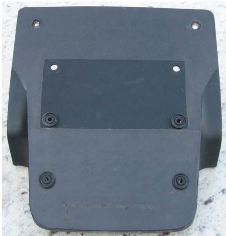
Figure 1. New mounting holes for license plate.
