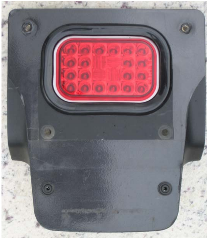
Figure 6. LED taillight installed in grommet.
