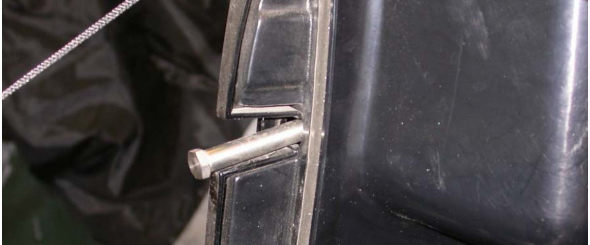
Figure 9: Taillight assembly bolt for 2004 and earlier LTs (10mm socket).
