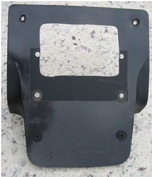
Figure 3. Hole cut for LED taillight.
