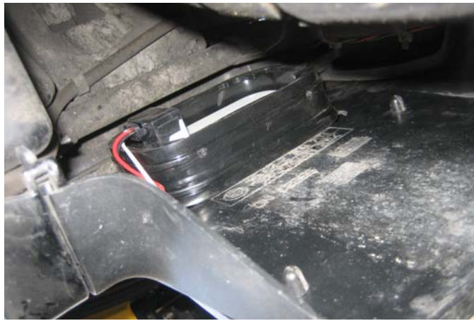
Figure 14. View from ground up, showing back of LED taillight.
