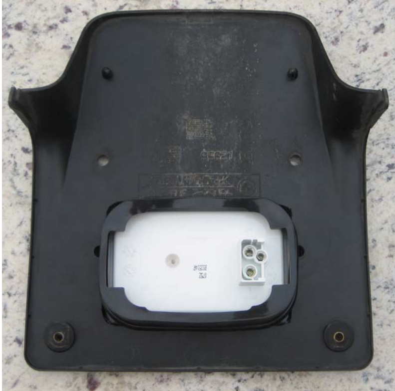
Figure 8. Back of license plate holder with LED taillight installed.
