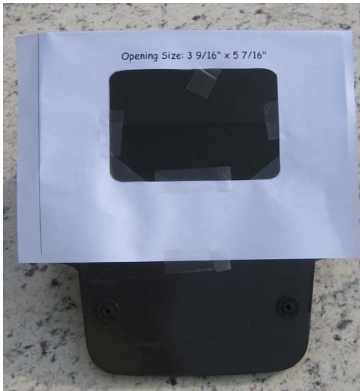
Figure 2. Template for LED taillight taped in place.
