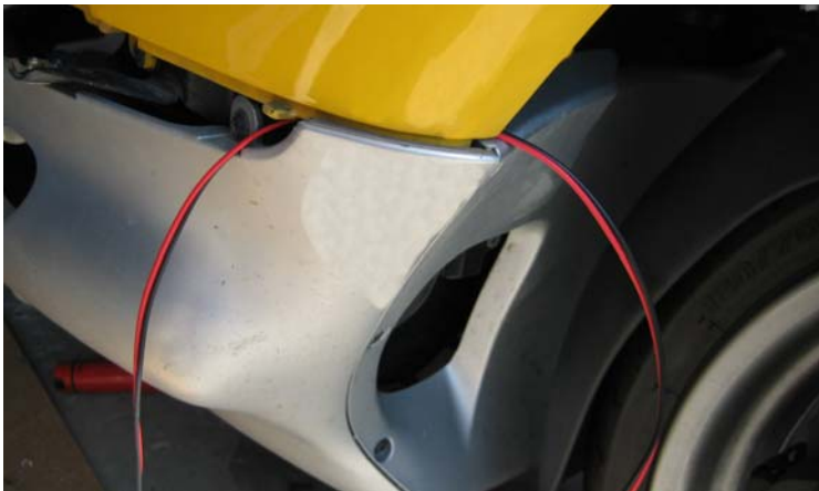
Figure 5: Running the wire from the nose of the bike to the tip-over wing
