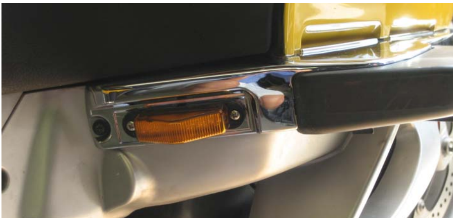
Figure 9: Tip-over wing with everything installed
