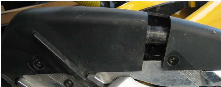
Figure 1: Screw locations on bottom of 2003 Tip-Over Wing cover (this cover is cut out for Bob's Highway Pegs). 2005 and later models have a courtesy light in the bottom of the cover.
