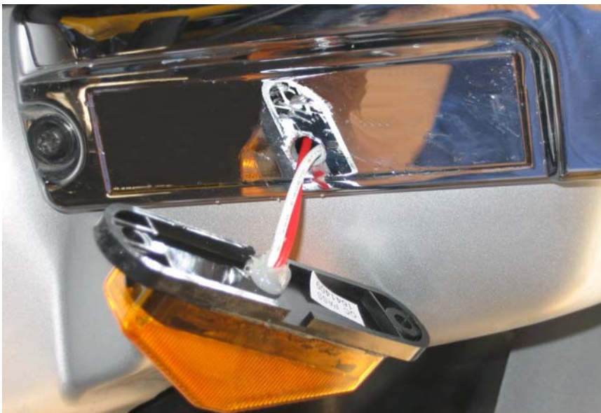
Figure 2: Location of the \frac{1}{4} " hole for the Marker Light wires
