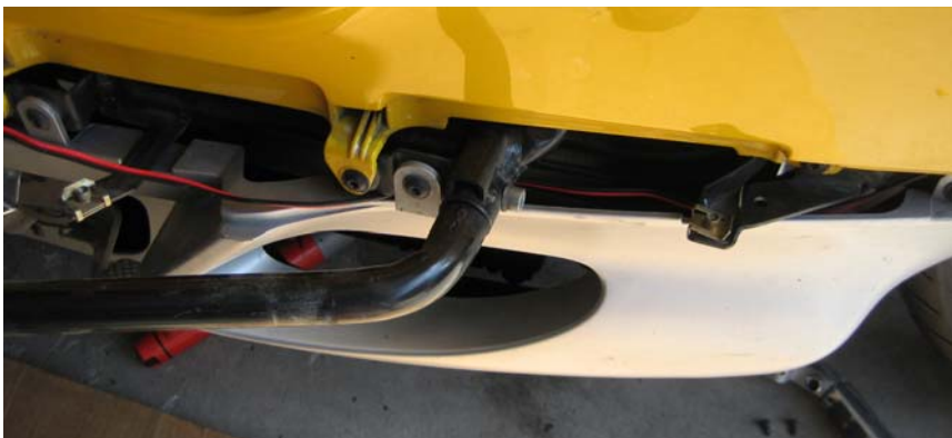
Figure 6: Running the wire in the tip-over wing
