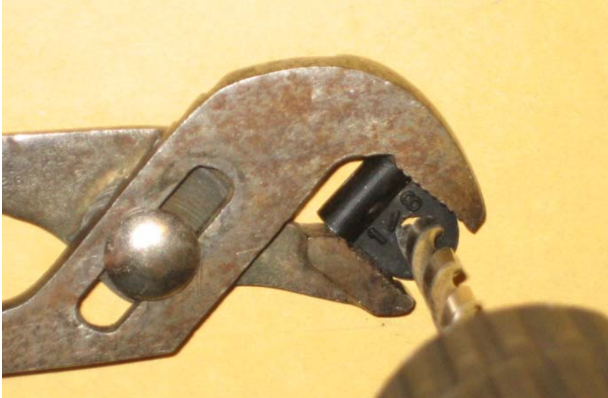
Figure 4: Drilling the hole larger in the cable clamp
