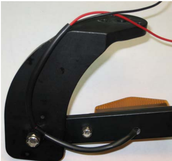
Figure 6: Wires secured to the backside of the Mick-O-Peg
