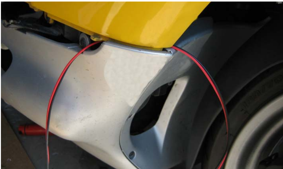
Figure 8: Running the wire from the nose of the bike to the tip-over wing
