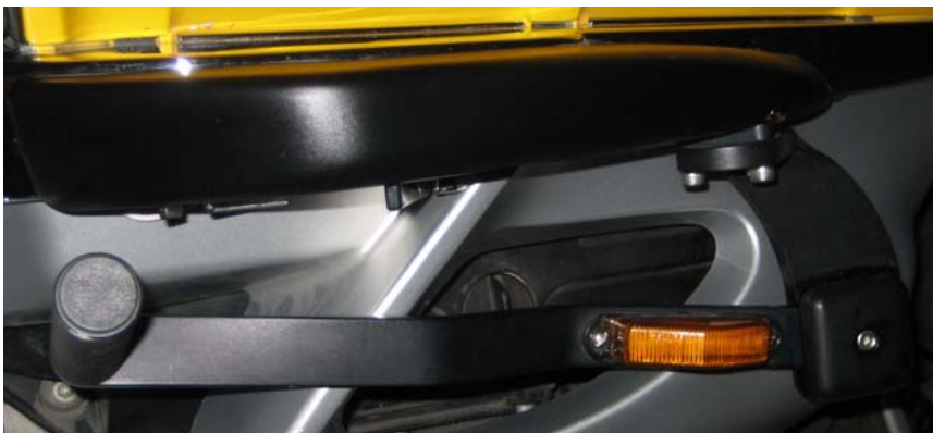
Figure 12: Mick-O-Peg installed with Marker light
