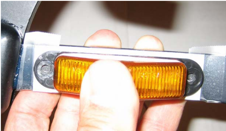
Figure 2: Test fitting the Marker light —note how the dots in the template align with the holes in the Marker light.
