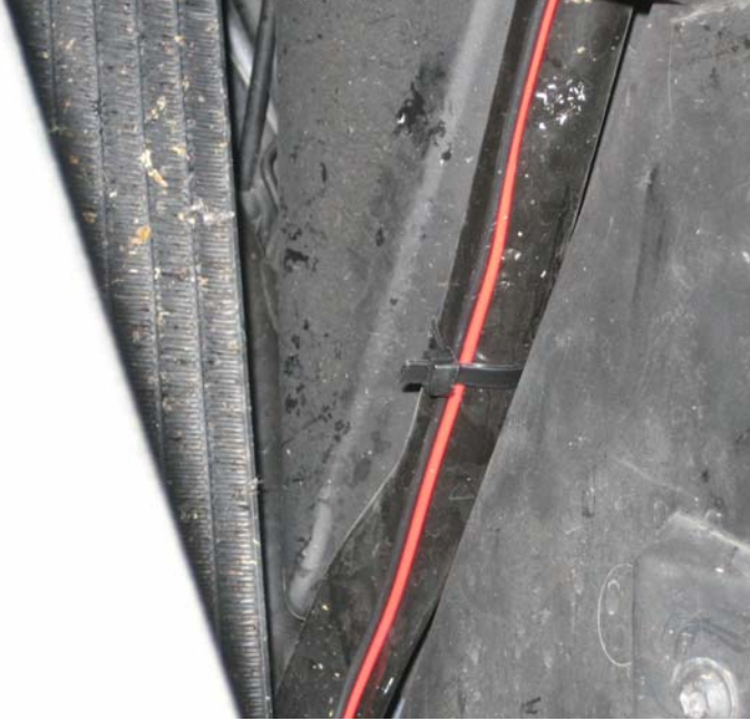
Figure 16: Zip cord secured with 7" black cable tie
