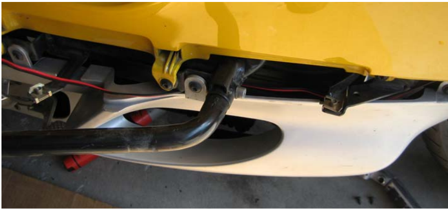
Figure 9: Running the wire in the tip-over wing
