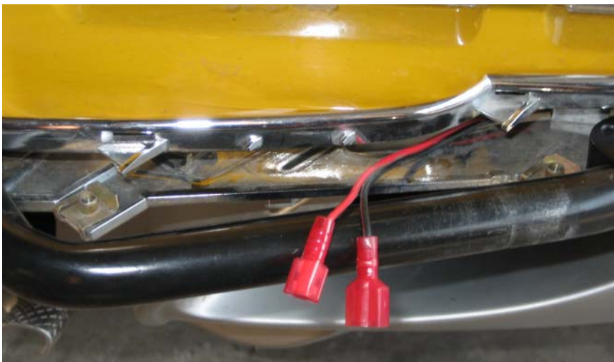
Figure 10: Connectors attached to wires going to nose of bike (shown with chrome cover replaced)
