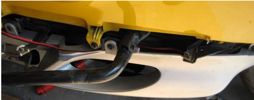
Figure 15: Running the wire in the tip-over wing
