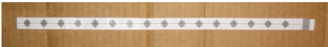
Figure 6: Drilling template taped together
