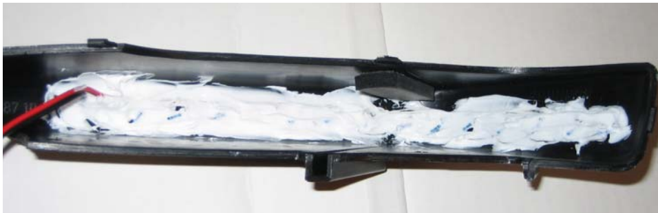
Figure 13: Inside of cover—LEDs and resistors are covered with silicon caulk
