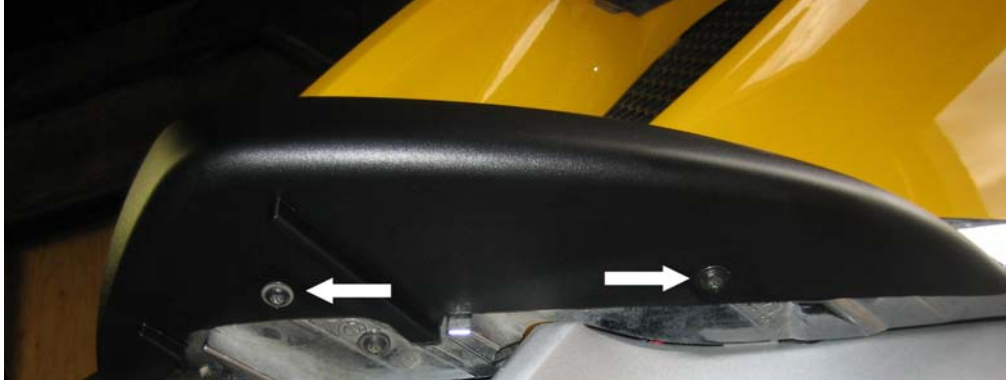
Figure 7: Screw locations on bottom of 2003 Tip-Over Wing cover. For 2005 and later models, you must also remove the courtesy light from the bottom of the cover.
