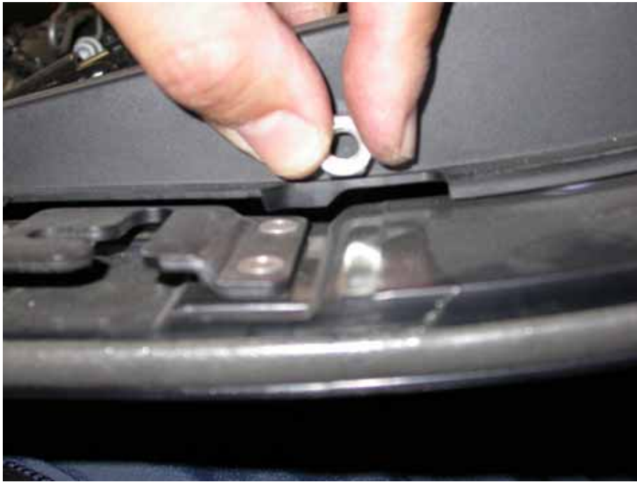
Figure 17. Marking the location for the pin switch
