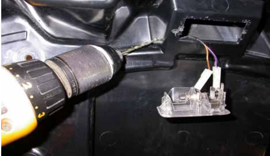
Figure 2: Drilling the hole for the wire
