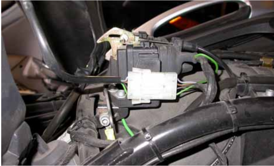
Figure 8. Connector for heated seat wires (viewed from left side of bike)
