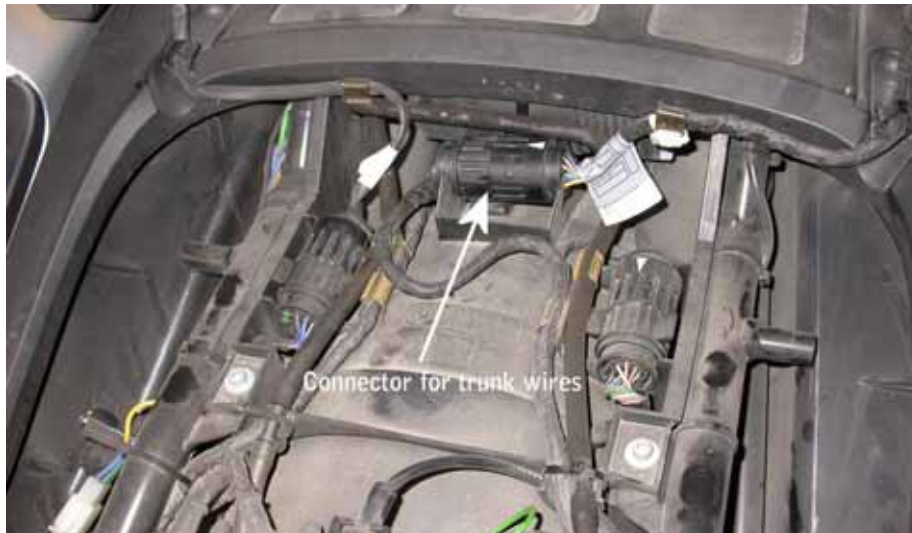
Figure 10. Connector for trunk wires
