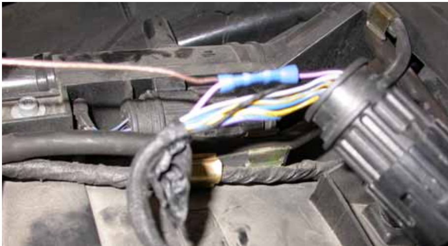
Figure 15. Blue butt connector attached to wires
