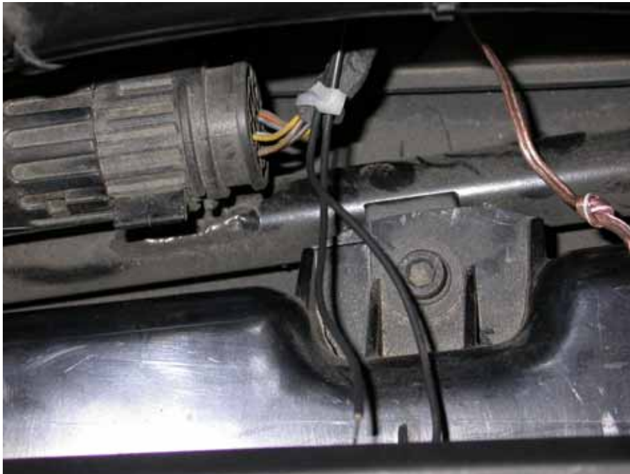
Figure 20. Pin switch wires secured to wiring harness
