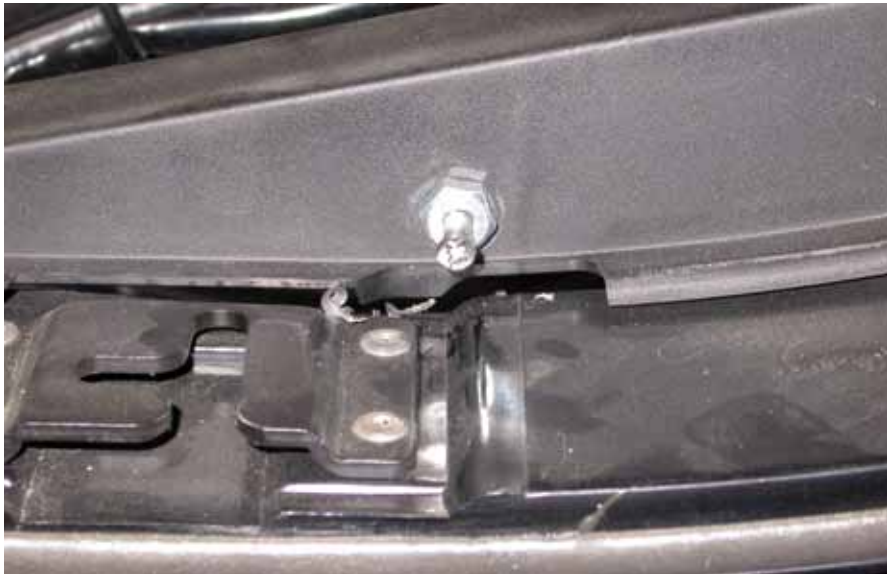
Figure 18. Pin switch installed
