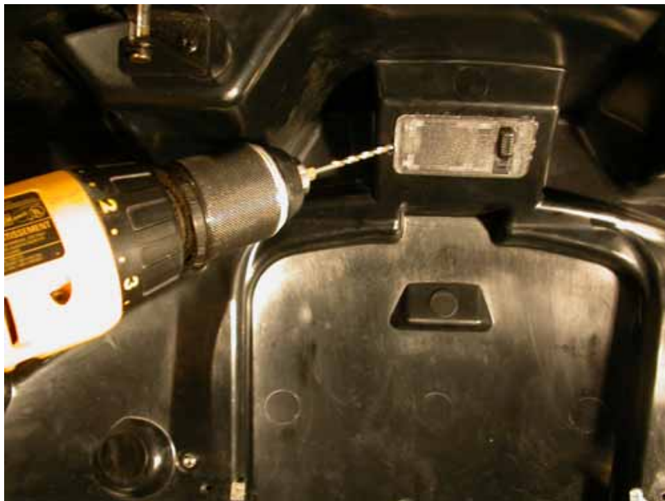
Figure 1: Drilling the release hole
