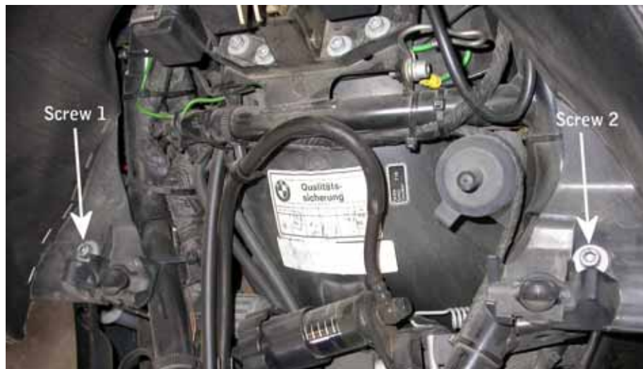
Figure 7. Remove two screws under the driver's seat to remove passenger seat (viewed from driver's seat facing back)
