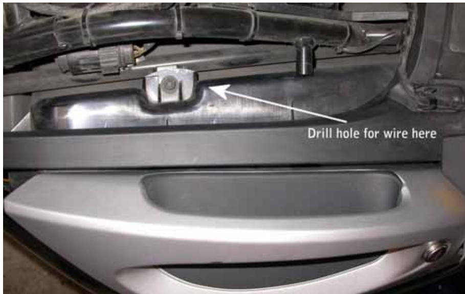
Figure 9. Location for drilling hole for wire (viewed straight down from left side of bike with saddlebag door closed)
