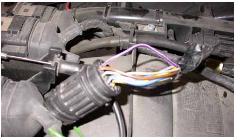
Figure 13. Purple wire for making "hot" connection
