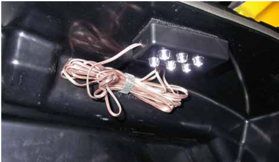
Figure 22. Light and wire bundle secured to top of saddlebag
