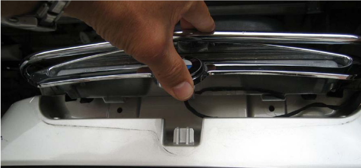
Figure 3. Removing the brake light assembly
