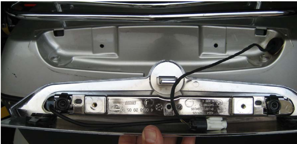
Figure 4. Note the tabs that help hold the brake light assembly in place
