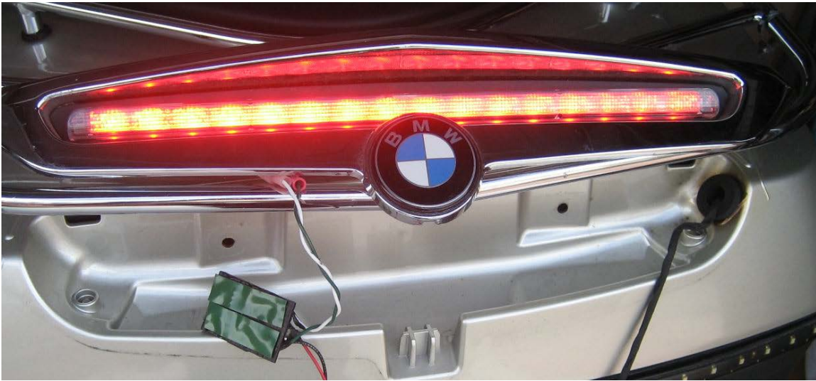
Figure 10. Successful test of the brake light flasher
