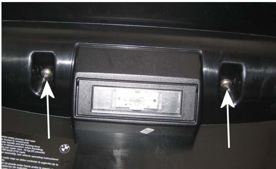
Figure 2. Removing the two screws to remove the brake light assembly
