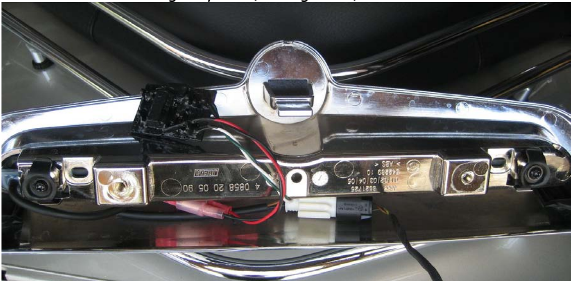
Figure 11. Tucking in all the connectors
