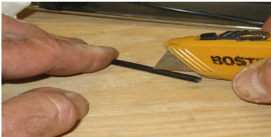
Figure 6. Cutting the insulation
