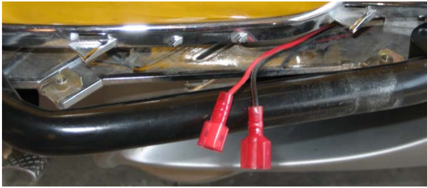
Figure 10: Connectors attached to wires in Tip-Over wing.
