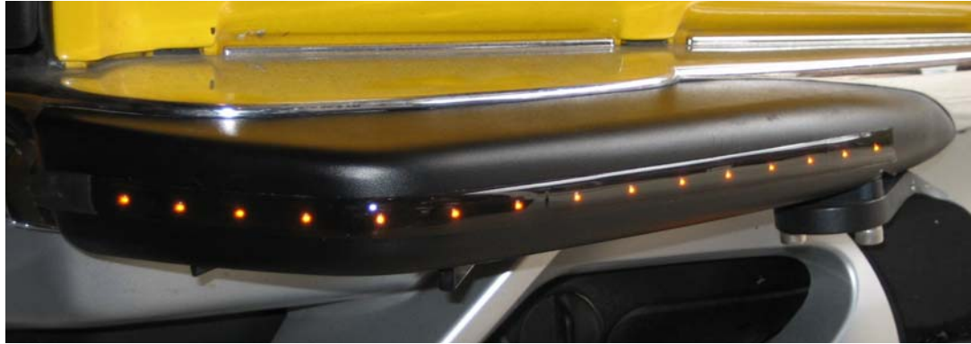
Figure 18: LED strip working.
