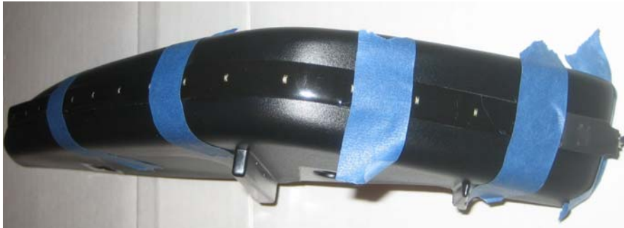
Figure 4. LED strip taped in place.
