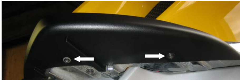
Figure 1: Screw locations on bottom of 2003 Tip-Over Wing cover. For 2005 and later models, you must also remove the courtesy light from the bottom of the cover.
