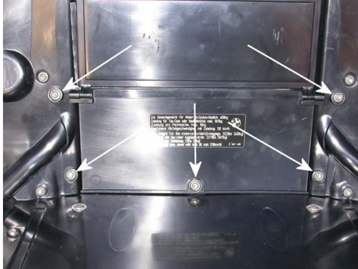
Figure 2. Remove 5 screws to remove plastic cover
